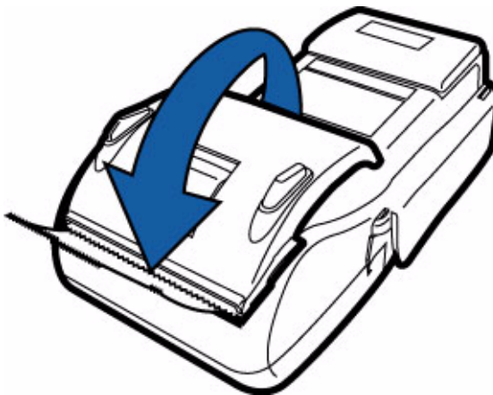
Figure 11 Closing Paper Roll Cover
