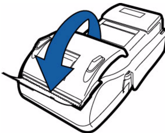
Figure 15 Closing the Printer Cover
